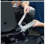
On Standard models, there are just nine daily grease points, Elite models having three extra on the high tip angle carriage. Every grease point is designed to be easy to access with remote greasing for those that would otherwise be difficult to reach.
