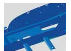
The one-piece H shape ladder chassis is made from 25mm thick, high tensile steel that is fully robot welded to ensure exceptional torsional rigidity. The boom support is exceptionally strong, its mass helping to counterbalance heavy loads.
