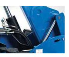
The boom hydraulic compensation cylinder is positioned to the rear of the boom and near the hinge point. The main lift ram is conventionally positioned under the boom. As the boom is raised both rams extend, but facing in opposite directions. This 'opposite working' helps to improve boom control, with additional benefits that include greater stability. The smooth action of the boom raise and lower reduces stress loads to enhance durability.
