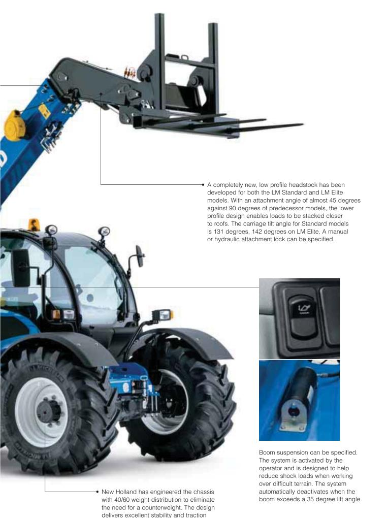
when loaded, the mass that would be used in a counterweight instead being built into the chassis to boost its strength.
