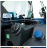
Access to the 140 litre fuel tank is via a wide opening filler, allowing in-field refuelling with cans if ever necessary. With a capacity of 27 litres, the AdBlue tank is large enough to last for at least 5 fuel tank fills.
